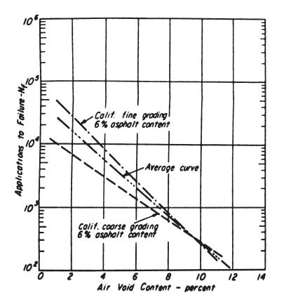
Figure 6. Influence of air void content on fatigue performance
