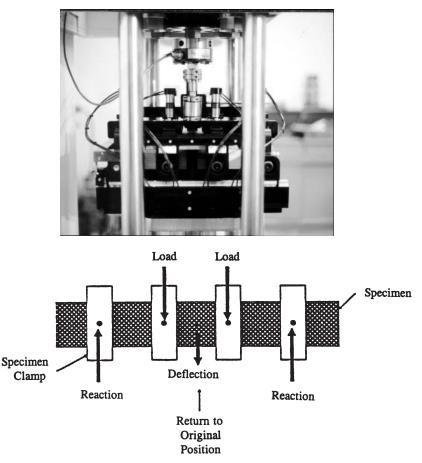
Figure 4. Schematic of third-point loading fatigue test apparatus
