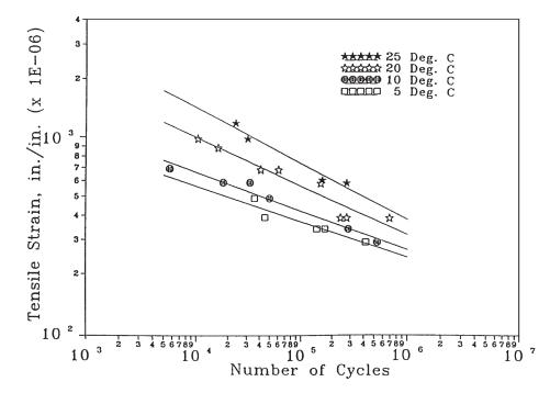
Figure 5. Strain-versus-fatigue relations for different temperatures
