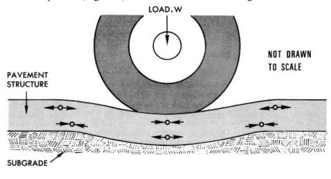
*Figure 2: Pavement deflection results in tensile and compressive stresses in pavement structure.*
