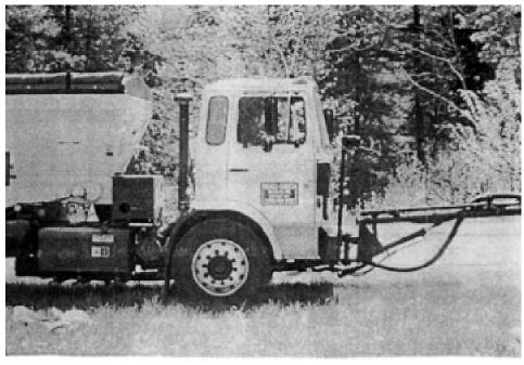
Figure 5. Spray injection device—self contained unit (photo SHRP-H-348)
