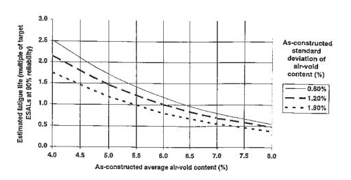
*Figure 3. Effects of as-constructed air-void content on pavement fatigue performance (chart from TM-UCB-CAL/APT-97-1)*
