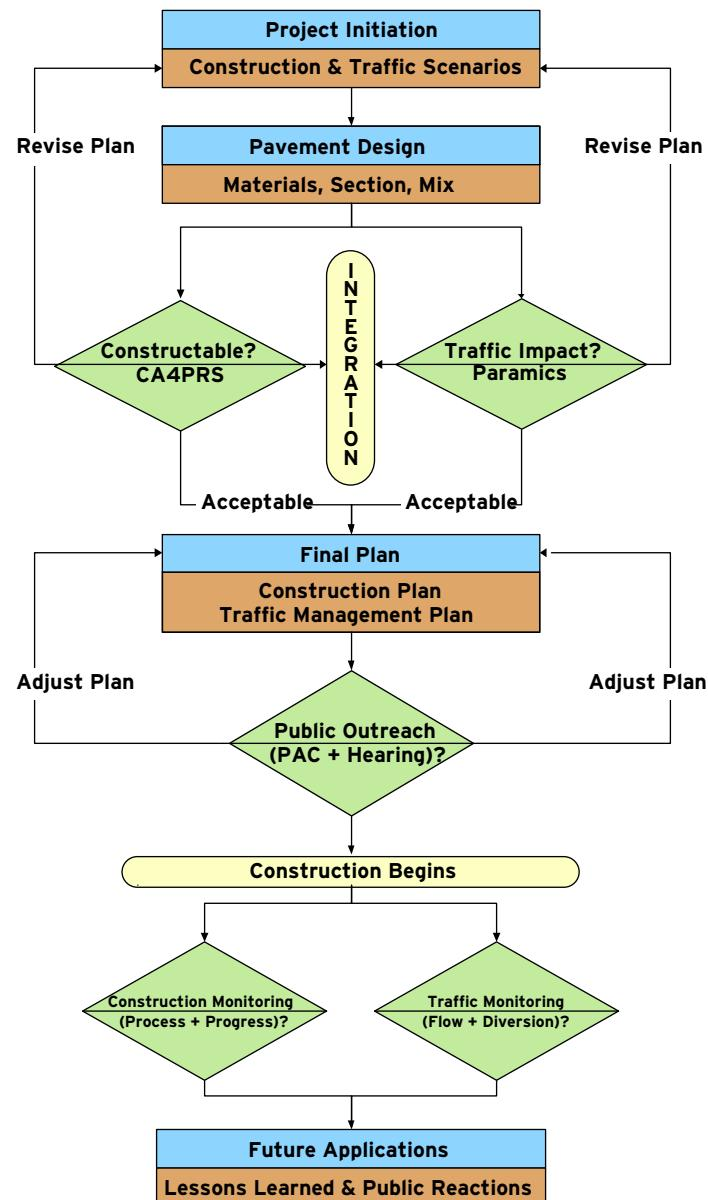
Framework for the integration of construction and traffic delay analysis for urban freeway reconstruction.
