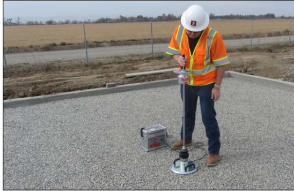
Figure 5.13: Light-weight deflectometer testing on the base.
