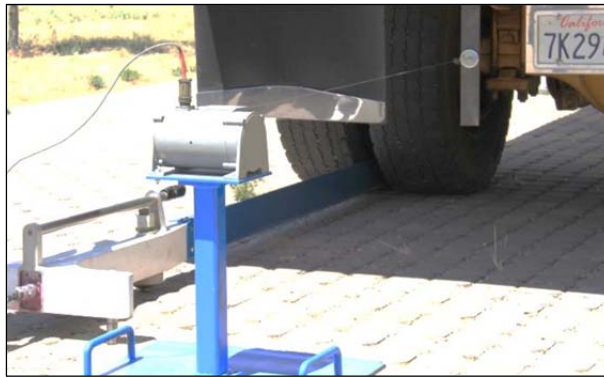
Figure 2.6: Encoder for measuring wheel location.
