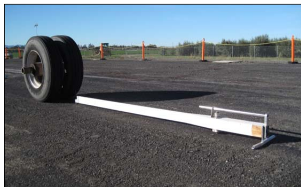
Figure 6.9: Road surface deflectometer.
