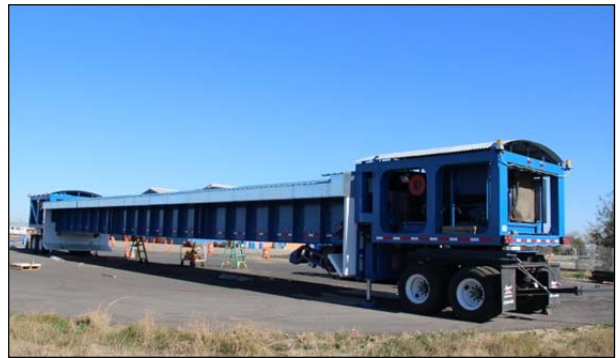
Figure 1.4: Heavy Vehicle Simulator with extended beam.
