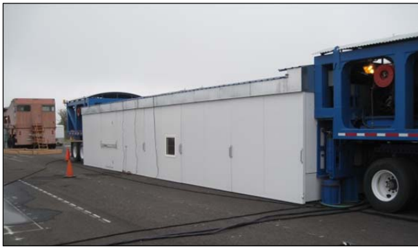
Figure 1.3: HVS with environmental chamber.
