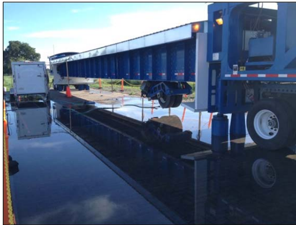
Figure 6.14: Flooded section during preparation for wet testing.
