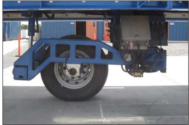
Figure 1.2: HVS test carriage.
